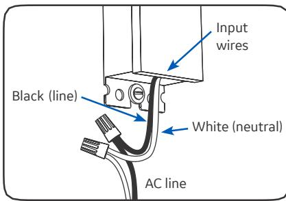
**2** Connect the AC line to the black (line) and white (neutral) input wires of the power supply using 18-14 AWG (0.82-2.08 mm<sup>2</sup>) twist-on wire connectors.
