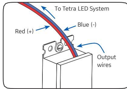
**3** Connect the supply wire that is attached to the Tetra LED System to the red (+) and blue (-) output wires of the power supply as outlined in the “**Electrical Connections**” section of your LED system’s Installation Instructions.
