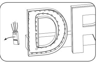
Remove the existing GECLPSPH. Do not remove existing channel letters and wiring.
