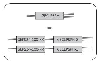
Two GECLPSPH-2 and two 24VDC, 100W, Class 2 Tetra LED Drivers will be required to replace each GECLPS5 or up to four GECLPS6 LED drivers.
