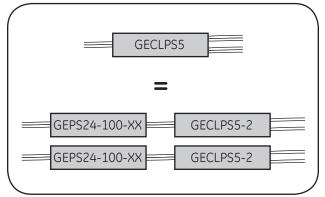
Two GECLPS5-2 and two 24VDC, 100W, Class 2 Tetra LED Drivers will be required to replace each GECLPS5 or up to four GECLPS6 LED drivers.
