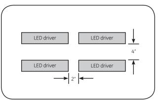
4 If installing multiple LED control modules or LED drivers in the same compartment, keep them at least 2" (50.8mm) apart end to end and 4" (101.6mm) apart along the sides.
