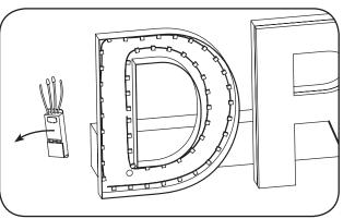
Remove the existing GECLPS5. Do not remove existing channel letters and wiring.
